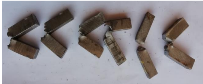
Fig. 4 Impact specimen after test.
